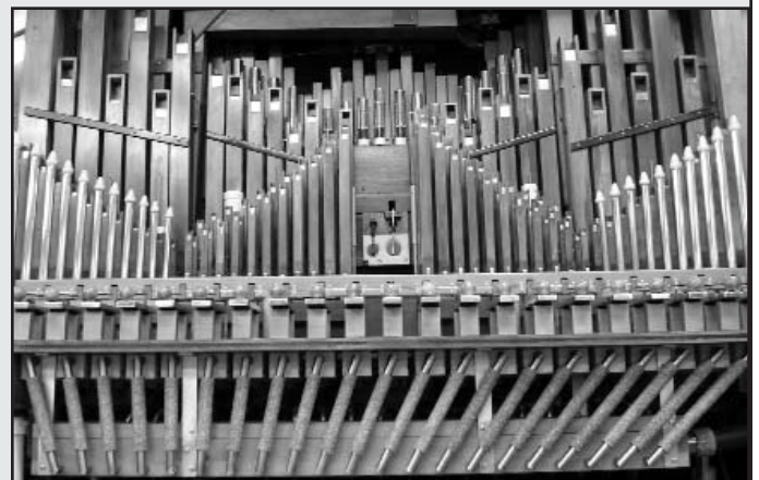
Figure 23. When the original bell action was removed is not known but there is evidence of such in the lower center section of the facade. An entirely new unit was fabricated in the Gavioli style and is shown attached temporary to the case by support legs. The bell action will be rejoined to the facade upon restoration completion.
