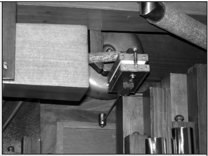
Figure 26. The brass bell illustrated is actually the fire bell effect from an American Photoplayer which was scrapped many years ago. It is taking the place of bell striking figures which may some day be added to this instrument.
