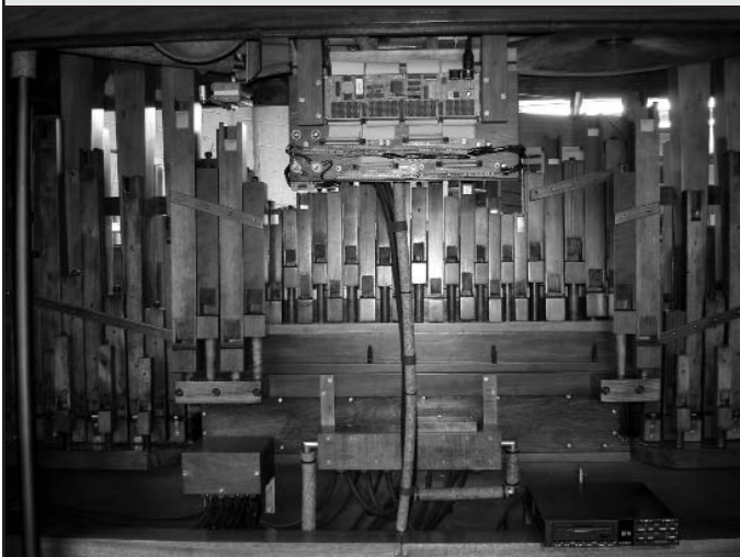
Figure 30. With the top back panel removed access is made to the MIDI decoder board. The Viscount media player can be seen in the lower right atop the magnet valve rail cover. An effort was made to hide the MIDI components and cables from view and make removal if desired simple. In fact it is estimated that all traces of the system could be removed in a few hours leaving only a few screw holes in the wake. Many thanks to Mike Ames and Ron Perry who provided MIDI components and understandable advice.
