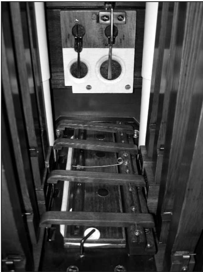
Figure 20 (left, upper). The lower unit is the four-stop Gavioli central register action with the clarinet register lock and cancel unit attached to the riser above. An additional register which controls the piccolo stop is located below the central unit and attached to the underside of the main chest.
