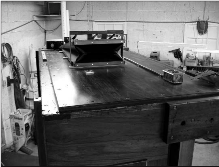
Figure 38. Topside view of the roof shows the added reservoir that enables the organ to play Wayne Holton's full arrangements without the need for over running the pumps. The hinge plate is used to fasten the skyboard of the facade. The 45 incandescent bulbs which are part of the facade plug into outlet boxes on each end of the case roof. The square box on the far left end is the DC power supply for the MIDI system.
