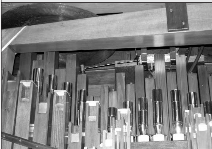
Figure 25. The crash cymbal and action fits as though Gavioli planned for one in the first place. It really adds to the music and other than a few screw holes no structural changes to the instrument were made.
