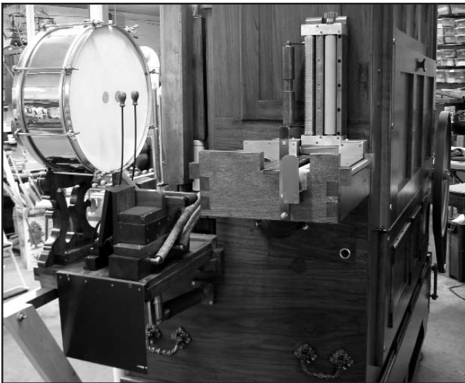
Figure 29. The completed keyframe in place and ready for book. In designing and building this unit, no particular brand of keyframe was faithfully copied. Instead it is a compilation of existing designs plus a few innovations. Once again, this builder is indebted to the late Ken Smith for his encouragement, advice, and sharing of printed materials for the fabrication of another keyframe.
