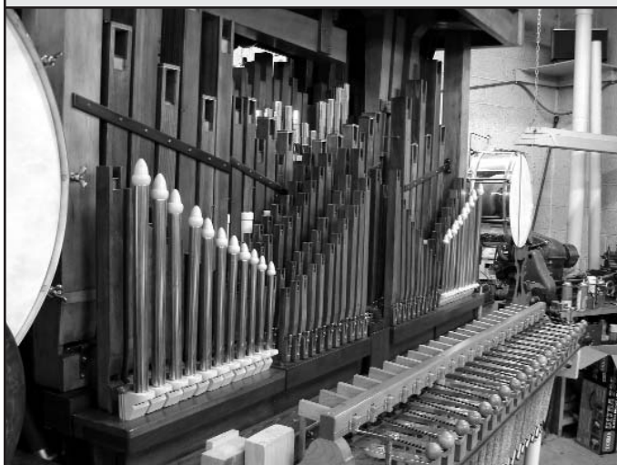
Figure 35. The brass panflutes were stripped of the black paint to find rose/pink as the original color which was matched and reapplied. Gold paint was removed from the brass pipe bodies and then buffed and lacquered. The panflutes and open harmonic flutes in this instrument have a distinctive and very powerful sound. There are no signs of any alterations having been made to these pipes in the past and are as the maker intended.
