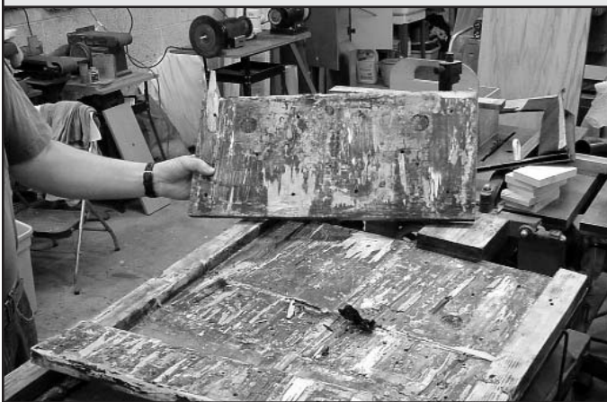
Figure 7 One never knows what lurks in the bowels of a band organ bellows. A well meaning repairman of the past made restoration of this pump a good challenge. Although many components needed to be made new, about 70% of the wood structure was made reusable. Any future rebuilds should be pleasurable.
