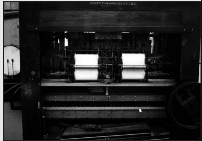
Figure 3. Backside of Savin Rock Gavioli shows duplex roll system for playing 66 key B.A.B. Rolls. After weighing the views offered to him by knowledgeable collectors, historians, and technicians, Gavioli owner Ken Harck made the decision to return the instrument to the basic design and intent of its' maker. Shortly after this picture was taken the roll system components were removed and declared surplus.
