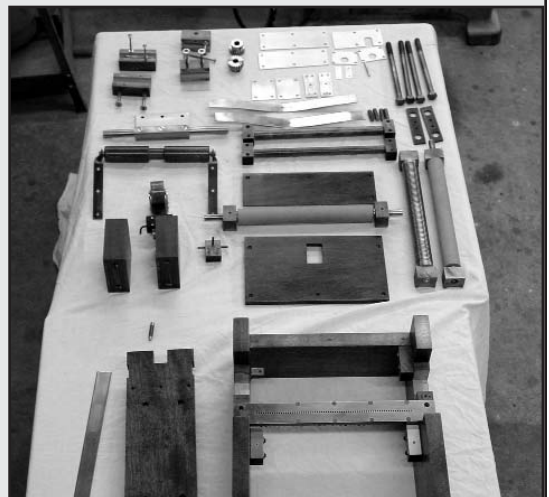
Figure 27. A 70 key(less) frame was fabricated to replace the long removed key(ed) frame that was fitted in the Gavioli factory. The basic wooden frame is shown in an early stage of construction. The wood is hard maple and the guide plates are stainless steel.
