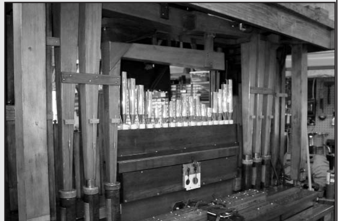
Figure 32. The six wood resonator trombones have a nice full sound without being “honky.” One hopes no problems develop with the reeds as access is difficult and requires removal of much pipework. For that reason special attention is made that reed wedges are installed securely.
