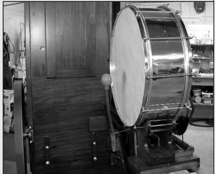
Figure 22. The bass drum beater motor in the inflated mode is connected to the cymbal striking action via a wood linkage. The valve activator motor can be partially seen directly under the drum shell. A badly worn and damaged cymbal was replaced with one of equal dimensions albeit new.
