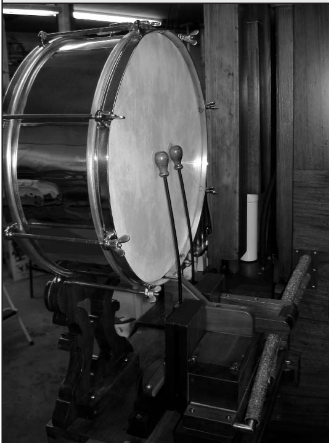
Figure 22. The bass drum beater motor in the inflated mode is connected to the cymbal striking action via a wood linkage. The valve activator motor can be partially seen directly under the drum shell. A badly worn and damaged cymbal was replaced with one of equal dimensions albeit new.
