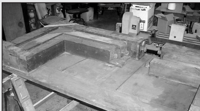
Figure 18. Bass bourdons mounted to floor of case before removal. Due to splits in mitered joints the pipes were mostly lifeless. A rodent nest was found in one pipe and nuts were in another.
